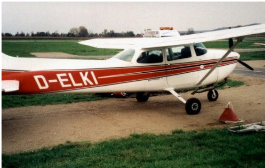
Cessna 172 N, Lycoming O-320-H2AD, 4 Zylinder, 160 PS
