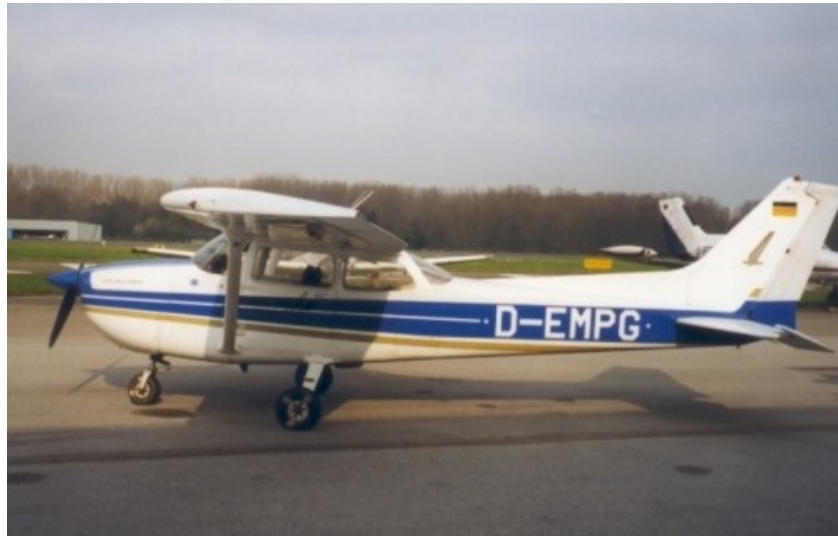
Cessna 172 N, Lycoming O-320-H2AD, 4 Zylinder, 160 PS
