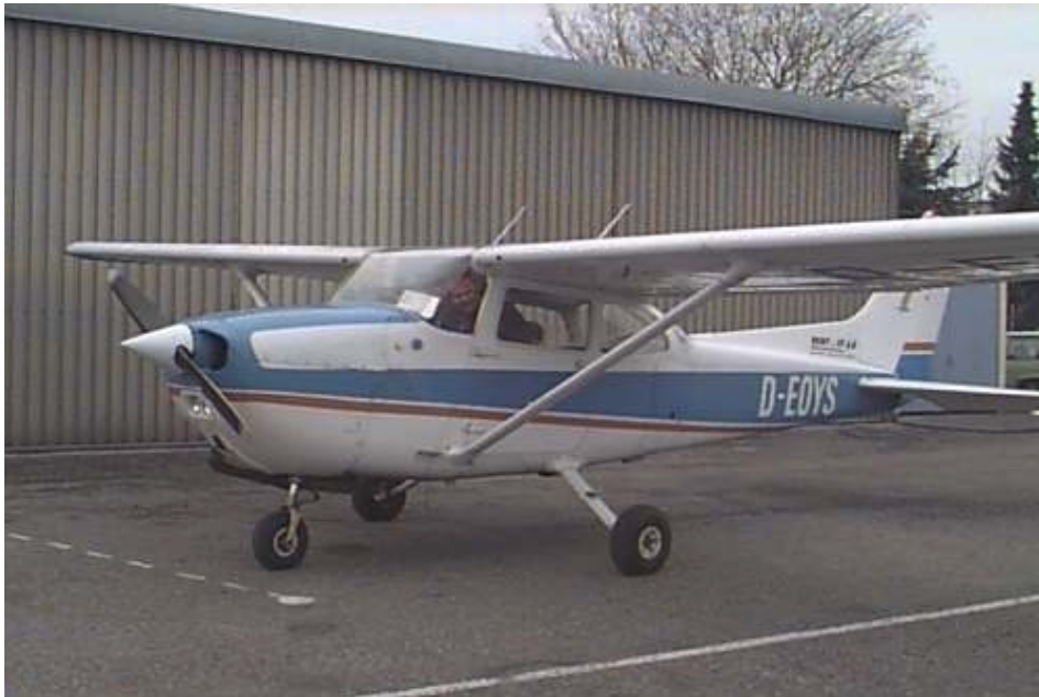
Cessna 172 N, Lycoming O-320-H2AD, 4 Zylinder, 160 PS
